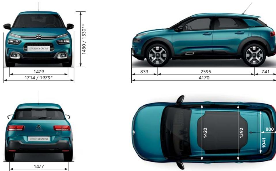
\* Vehicle width/width with side mirrors out. \*\* Height with roof bars.
