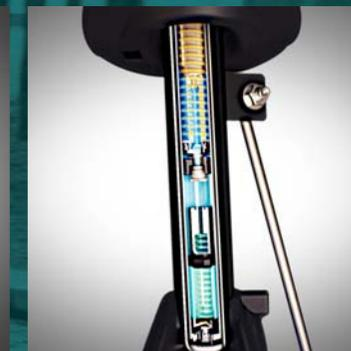
*On light compression and rebound, these hydraulic cushions provide a "flying carpet" effect by erasing the roughness of the road.*
